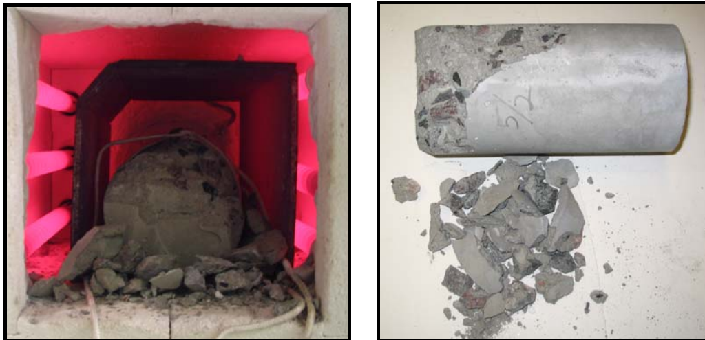
(a) Spalling Failure under different surface temperatures, T_{\text{surf}}=400 : WF_400_1
