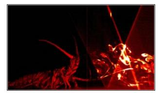
Researchers are using robots to solve the mystery of "lobster sniffing." Here, a plume of fluorescent dye, illuminated by a sheet of red laser light, floats towards the robotic lobster at a rate of 10 centimeters per second. The olfactory antennule is extended in front of the lobster. Photo courtesy of: Megan Wiley, Jeffrey Koseff and Mimi Koehl
