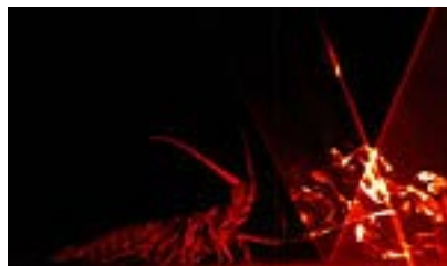
CAPTION: A discarded lobster shell fitted with a motor-operated antennule that mimics the flicking used by lobsters when they sniff. A laser illuminates fluorescent dye in the turbulent water, allowing scientists to study how odors penetrate the lobster's nose. Credit: Mimi Koehl/UC Berkeley, Meg Wiley & Jeffrey Koseff/Stanford
