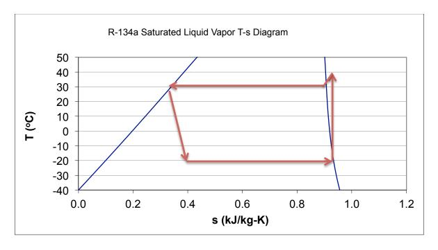
18. Calculate the work input to the compressor (kJ/kg). (You do not need to interpolate, you may round the entropy value at the compressor inlet to 3 significant figures.)
